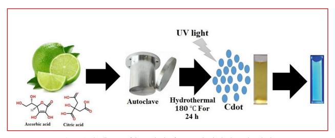
Figure 1. The diagram of the synthesis of CQDs using hydrothermal methods
