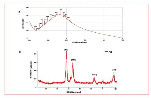
**Figure 3A.** UV-visible absorption spectrum of AgNPs synthesized using *N. officinale* leaf extract treated with 10mM AgNo<sub>3</sub>.
