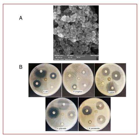
**Figure 4.** A SEM micrograph showed the morphology of synthesized AgNPs using N. officinale leaf extract.
