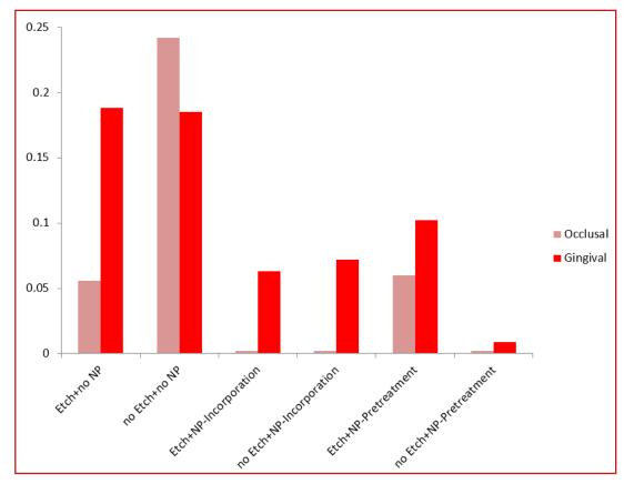
Chart 2. The mean of microleakage in the occlusal and in the gingival. Tio<sub>2</sub> NPs in both total-etch and self-etch approaches led to a decrease in the microleakage. Kruskal-Wallis test showed significant differences in the microleakage of occlusal margins (P<0.001) but in the gingival margins, we did not any significant differences (P=0.128)
